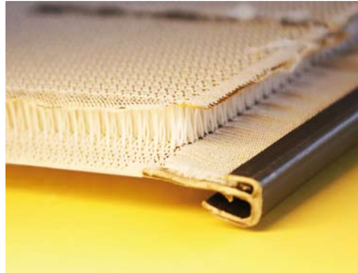
3D - Woven Fabric, 20 mm thick showing the bent shape of the pile fibers after weaving. The rigid fibers provide pressure stability.
